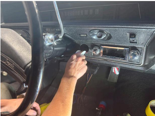
Now feed the cable through the hole and insert the display. Make sure to orient the opening downward to keep the correct orientation of the display when powering it on.
