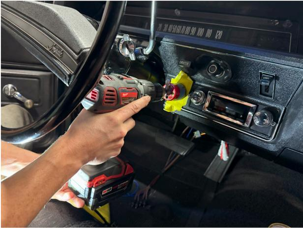
Locate where you plan on installing the Display and tape it off. To drill the hole use a 1 3/4" hole saw to drill the opening.
