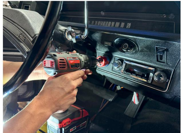
Next sand the opening in order to make room for the display as it is a little larger than 1 3/4". Be sure not to sand too much as the display should have a snug fit.
